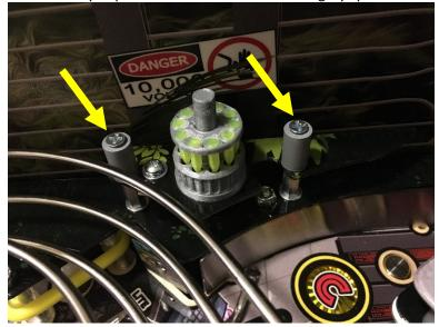
7. Install the can on top of the base using a back and forth twisting motion (the fit will be very tight, so you will want to give support from underneath the plastic with pressing down on the can. The bottom of the can should be just above or cover the silver ring that supports the vials. The mod fits pins with and without Pin Stadium lighting, so you will want to test fit with light bars installed if you have them. Just adjust the can height as needed.
