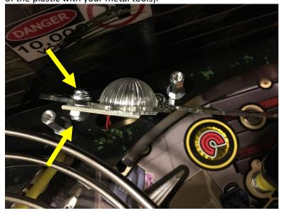
4. Insert the base of the mod up through the bottom of the plastic just as the clear dome was installed, align the tab hole with the hole in the plastic, and put screw/washer in hole from the top.
