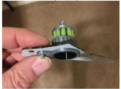
5. Place flasher board onto screw, and replace locknut. With the flasher bulb centered below the opening in the base, tighten the screw while holding the nut with pliers.
