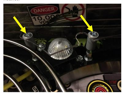
3. Pull out remaining assembly being careful not to overstretch with attached wires. Pay attention to how everything is ordered on top and bottom of the plastic as you will reassemble the same way. Remove the screw holding the dome and flasher in place using pliers to hold the nut (be careful not to scratch any of the surfaces of the plastic with your metal tools).
